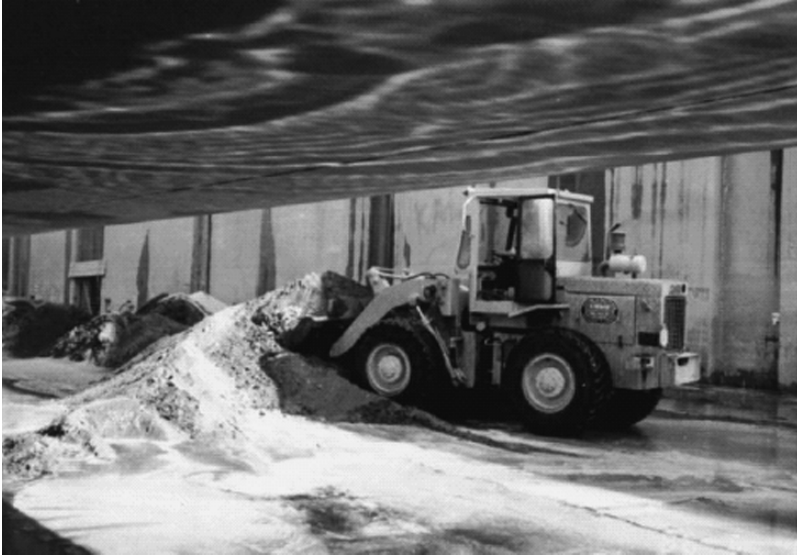
Fig. 7.26 Solid waste to be dealt with after blast cleaning of a ship construction (Photograph: Lightgow Assoc.)
