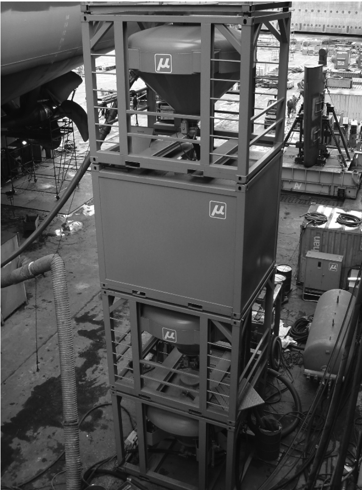
Fig. 7.29 Mobile abrasive recycling unit for large-scale applications (Photograph: Muehlhan AG, Hamburg)
