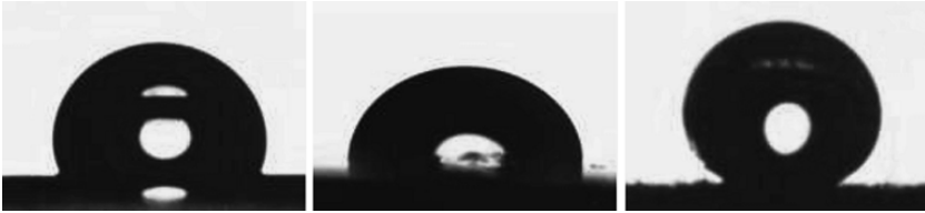
Fig. 8.72 Effects on contact angle formation (Fraunhofer Society, München). Conditions: left – initial condition; centre – effect of roughness; right – effect of contamination
