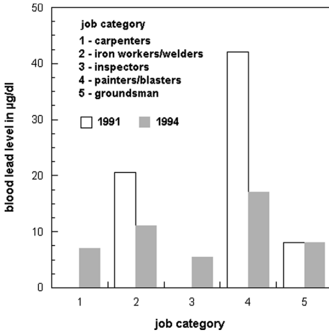
Fig. 7.16 Blood lead levels for bridge workers (Maurer et al., 1995)
