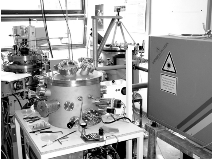
Fig. 7.3. View into the PLD lab of the author in the Semiconductor Physics Group (head M. Grundmann) at University Leipzig, with three PLD chambers, excimer laser Lambda Physik LPX 305, and optical laser beam guiding system inside protection shielding. Two more PLD chambers are in the neighboring lab to the right
