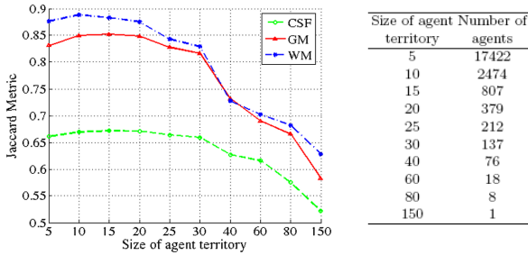
Fig. 5. Influence of tissue agent territory size on the robustness to intensity nonuniformity, using the BrainWeb phantom with 3% of noise and 100% of nonuniformity
