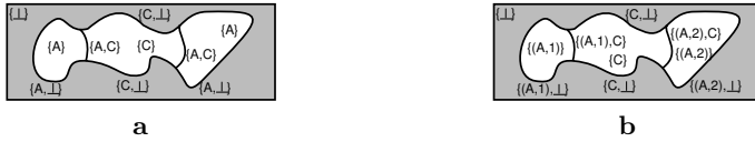
Fig. 3. Figure a shows a spatial partition with two regions and its boundary and region labels. Figure b shows the result of the refine operation on Figure a .
