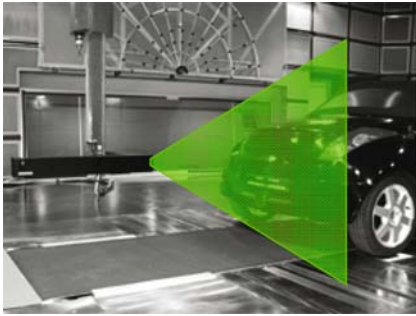
Fig. 4. Experimental setup to measure the three velocity components of the flow in the near-wake region of a test car in the Pininfarina full-scale automotive wind tunnel. The Pininfarina probe is mounted on the main traversing system. The image of the laser lightsheet is shown for the sake of clarity
