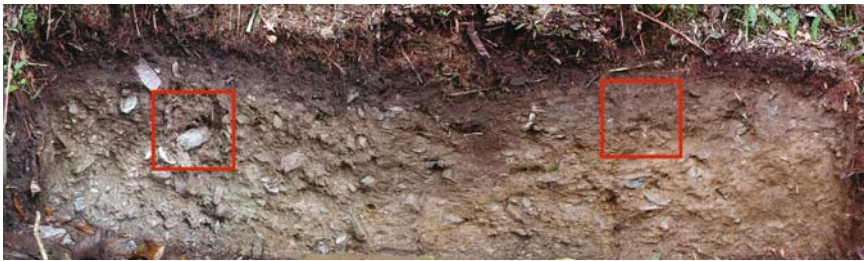
Fig. 30.1 Photograph of a 4.0×1.5 m soil profile. The red squares show two digitized sections used for water flow simulations. Photograph by J. Zeilinger
