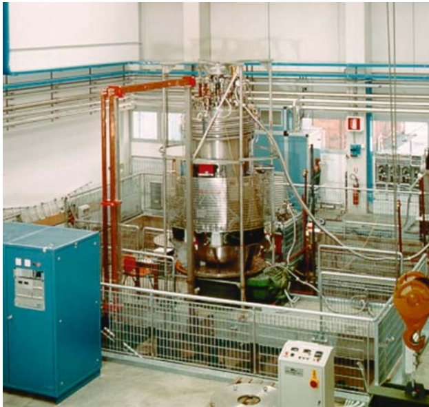
Fig. 9.7. View of the cryostat with the magnet inside during assembly. The cryostat is mounted on a turntable fastened to a concrete beam spanning the PVLAS dugout. The turntable is situated below the cryostat. The magnet power supply is the cabinet visible at lower left
