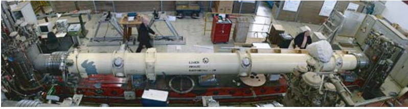
Fig. 10.12. Superconducting HERA dipole magnet exploited by ALPS for conversion of laser photons into axion-like particles, as well as for the reconversion of axion-like particles into photons
