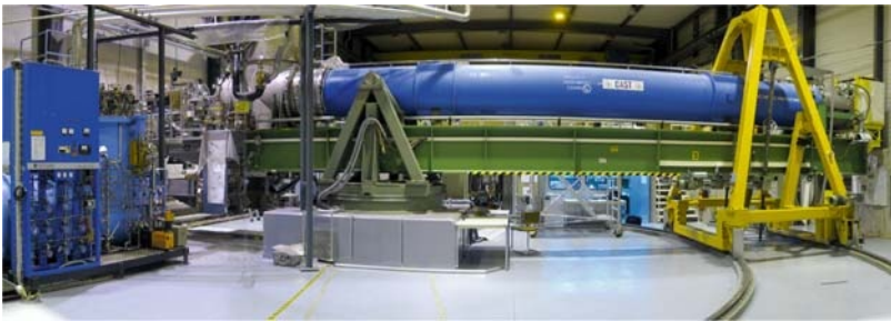
Fig. 10.5. Experimental setup of the CAST experiment at CERN. From the left to the right the Helium cryogenic system, the CAST superconducting magnet, and the tracking system is shown. The tracking system allows to follow the Sun 1.5 h per day during sunrise and sunset
