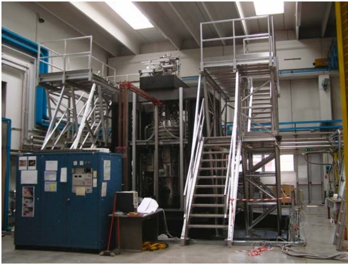
Fig. 9.9. View of the PVLAS granite tower and of its aluminum access structure. The cabinet visible at lower left is the magnet power supply
