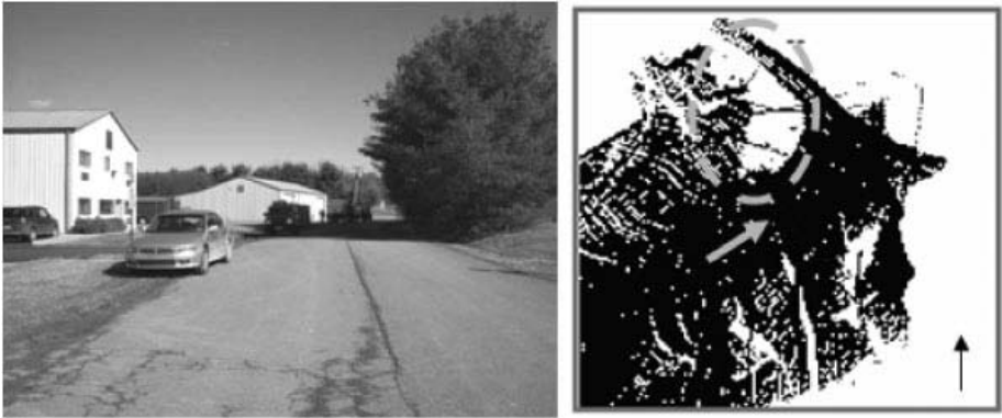
Fig. 5.11. The image on the left shows a parked car from Rocky's point of view. The image on the right shows scanned terrain colored black. The position and orientation of Rocky is denoted by the grey arrow. A parked car blocks LADAR scans, leaving an unscanned shadow, circled on the right image.
