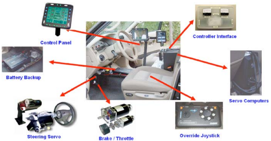
Fig. 15.2. EMC provided the drive-by-wire capability using a steering servo, a throttle/brake servo, a control console, two servo computers, a battery backup, and a manual override
