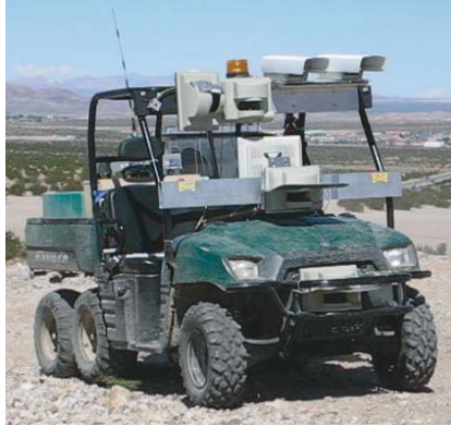
Fig. 6.1. Vehicle ION: the Intelligent Off-road Navigator. The vehicle is a 2005 Polaris Ranger 6x6. It is 120 inches long and 60 inches wide and its height is 78 inches. Drive by wire capability has been added to the vehicle so that computer control is possible for throttle, brake, steering control, and transmission gear switching.
