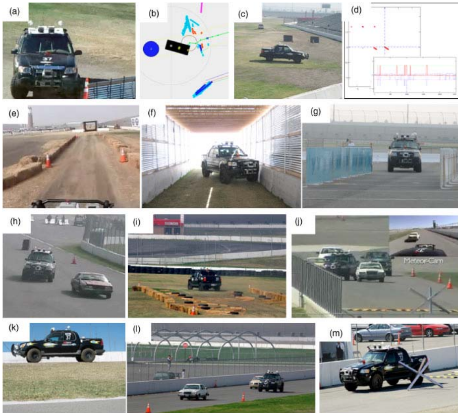
Fig. 15.15. NQE. Each team had six chances to complete the course. a,b) Meteor's first run ends as it fails to pass through the first gates. c,d) Meteor veers off course before reaching the gates. e,f,g) During the third run, Meteor clears the gate, rounds a steep hill and traverses a hay bale maze, but stops in the tunnel. Testing corrected this discrepancy. h-m) Meteor completes runs 4, 5 and 6 without incident, including avoiding several parked cars, a debris field, a mock mountain pass and a tank trap. Completing three runs qualified Meteor for the finals.
