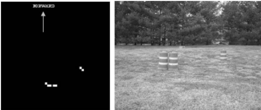
Fig. 5.13. The local cost map (top-down view, left) generated by the horizontal LADAR for a typical scene with obstacles (vehicle view, right)
