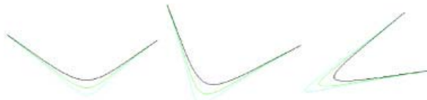
Fig. 12.15. Candidate cubic paths generated for various turns. The paths are constructed from pairs of control points at the beginning and end of the path. Families of cubics are generated by varying the spacing of the two center control points.
