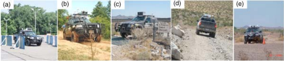
Fig. 15.14. Testing. a) Most vehicle testing occurred in an empty parking lot in McLean, Virginia. Here Meteor passes through a mock tunnel constructed from wood and weather tarps. b) Testing at local sites including a farm and an off-road facility. Note deep ruts that proved hazardous to low lying sensors. c) Six days of testing in 129 degree heat of Primm Nevada in July. Here Meteor successfully exits a tunnel and passes through cattle guards. d) Testing along the 2004 route included driving in rough mountain terrain. Note the size of the boulders left of Meteor. e) Testing on an off-road autonomous vehicle test course at the Yuma Proving Grounds a week before the race.
