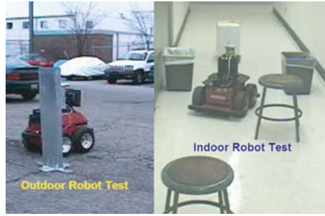
Fig. 6.13. Test obstacle avoidance algorithm on small robots. We used an all-terrain-robot-vehicle (ATRV) for outdoor tests and a PIONEER P3-AT robot for indoor tests.
