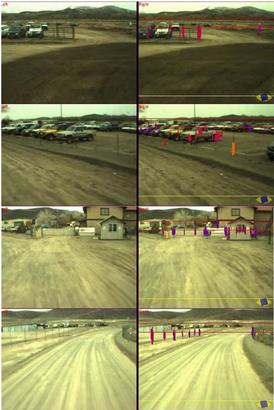
Fig. 4.14. Images showing left and right images of different situations; on the right images, colors show the presence of detected obstacles: different colors mean different distances. The additional horizontal lines represent the 5m, 50m, and horizon position. Posts and thin poles as well as fences posts are correctly detected.
