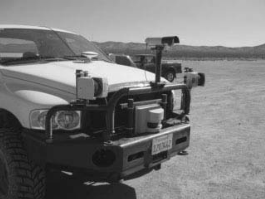
Fig. 7.17. The camera is mounted inside a housing atop a pole connected to the front bumper. This allows a better field of view than mounting the camera on the windshield.
