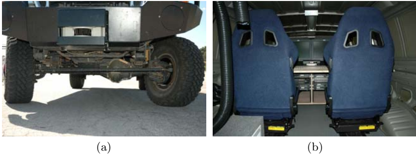
Fig. 14.2. Vehicle features: (a) front differential, suspension, and front bumper/LADAR mount and (b) the rear workstation area with server array visible (as viewed through the rear doors)
