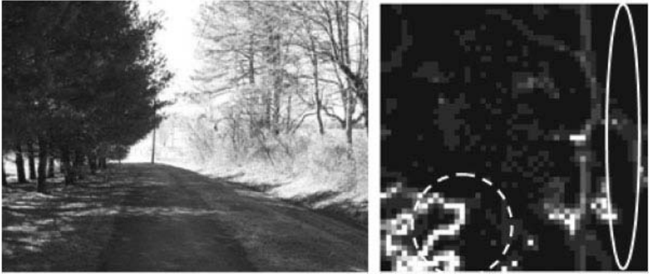
Fig. 5.16. Typical LADAR overlay map of sensor data for the Virginia Tech Grand Challenge A* graph search (right). Dark shades indicate areas of low cost, while light areas indicate areas of high cost. The area enclosed in the white oval indicated a significant drop off; the area circled in dashes indicates the trees pictured at left.
