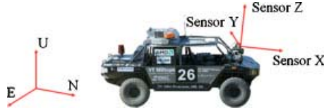
Fig. 13.9. Example sensor axes and ENU reference axes that determine the transformation from sensor to terrain measurements
