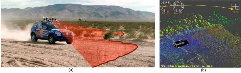
Fig. 1.7. (a) Illustration of a laser sensor: The sensor is angled downward to scan the terrain in front of the vehicle as it moves. Stanley possesses five such sensors, mounted at five different angles. (b) Each laser acquires a 3-D point cloud over time. The point cloud is analyzed for drivable terrain and potential obstacles.
