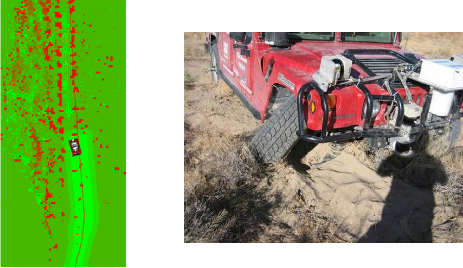
Fig. 2.22. An example of incomplete data (a) which led to significant damage (b). The red continuous line represents the pre-planned path. The data shows that the pre-planned path is on the road edge and veers off the road, which combined with the with the hill crest to cause the robot to leave the road.
