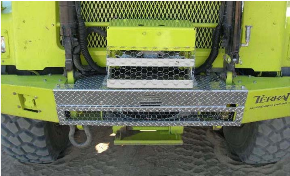
Fig. 4.12. The front of the TerraMax vehicle. Two 4-plane laserscanners are visible; The one inside the bumper is the one used during the race, the other (over the bumper) is a backup.
