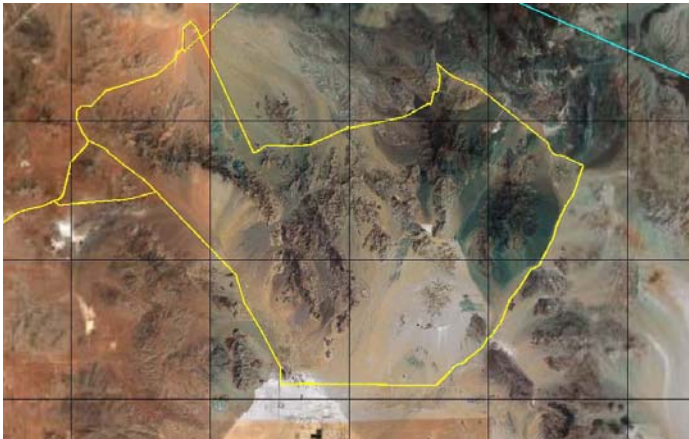
Fig. 14.19. A compilation of several RDDFs used during testing within the Stoddard Wells area of the Mojave Desert. The grid lines are 10 km apart. The RDDF leaving the top of the figure is the 2004 race RDDF, and the line cutting across the top right corner is the boundary of the no-go zone given by DARPA. These RDDFs covered a wide variety of desert terrains, including dirt roads, rocky hills, dry lake beds, bumpy trails, smooth pavement, and mountain passes. During the majority of testing the RDDF speed limit over the entire RDDF was set to be unlimited, and the vehicle’s speed was chosen automatically as it traveled.
