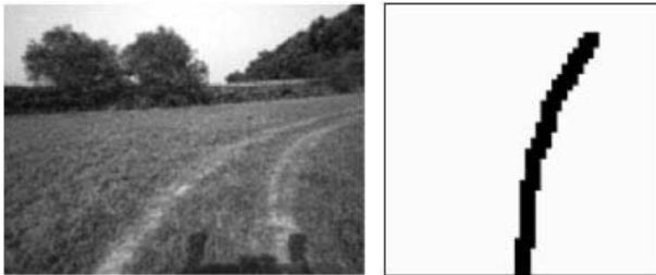
Fig. 5.14. The recognized road from the RGB image (left) is translated into a local road map (right)
