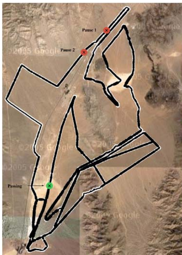
Fig. 1.27. This map shows Stanley's path. The thickness of the trajectory indicates Stanley's speed (thicker means faster). At the locations marked by the red 'x's, the race organizers paused Stanley because of the close proximity of CMU's H1ghlander robot. At Mile 101.5, H1ghlander was paused and Stanley passed. This location is marked by a green 'x'.
