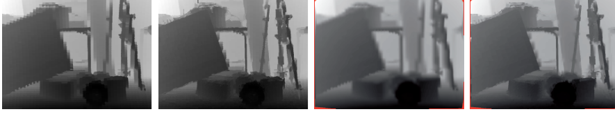
Fig. 10.2. From left to right : Depth image generated with the NR method. Depth image generated with the NRC method, small details are now visible, note that a depth image generated from a similar viewpoint as the laser range scanner makes it very difficult to see flaws of the interpolation algorithm. MLI method. LIC method
