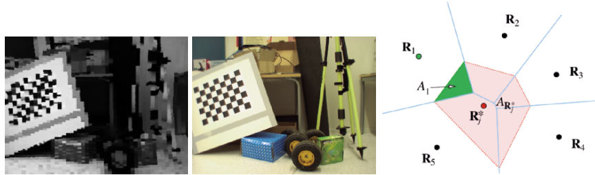
Fig. 10.1. Left: Image intensities plotted with the resolution of the 3D scanner. The laser range readings were projected onto the right image and the closest pixel regions were set to the intensity of the projected pixel for better visualisation. Middle: Calibration board used for finding the external parameters of the camera, with a chess board texture and reflective tape ( grey border ) to locate the board in 3D using the remission/intensity values from the laser scanner. Right: Natural neighbours R_1 \dots R_5 of R_j^* . The interpolated weight of each natural neighbour R_i is proportional to the size of the area which contains the points Voronoi cell and the cell generated by R_j^* . For example the nearest neighbour R_1 will have influence based upon the area of A_1
