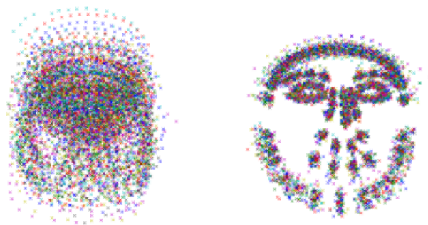
Fig. 6. Key facial points plots before/after the Procrustes Analysis. Left: before, Right: after.
