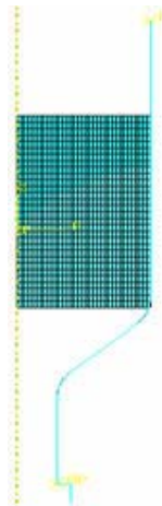
Fig. 4. FEM model for the micro extrusion
