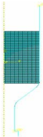
Fig. 4. FEM model for the micro extrusion
