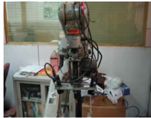
Fig. 1. Binocular vision system used in this paper
