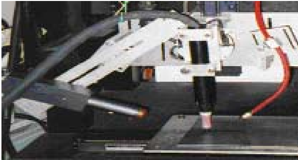
Fig. 1. Close-up of the arrangement of strobe imaging sensor (left), TIG welding torch (centre) and the laser illumination (right)
