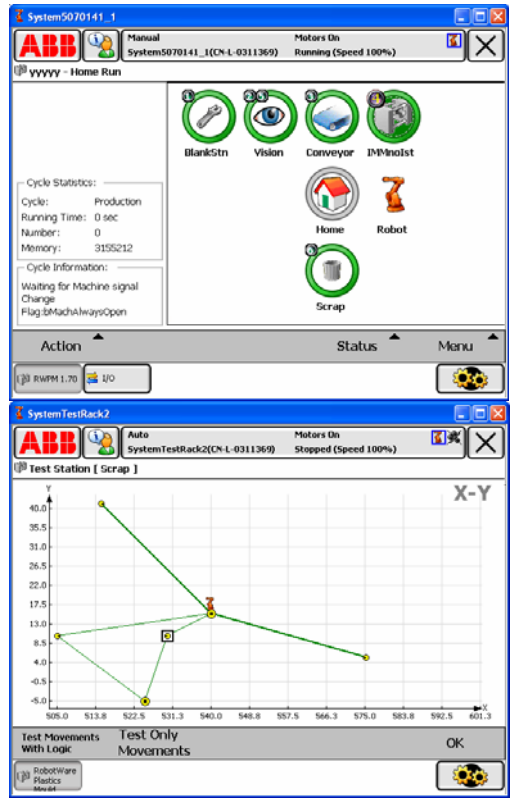
Fig. 4. GUI design (a) Intuitive representation of work cell layout (b) 2D map of robot tracks
