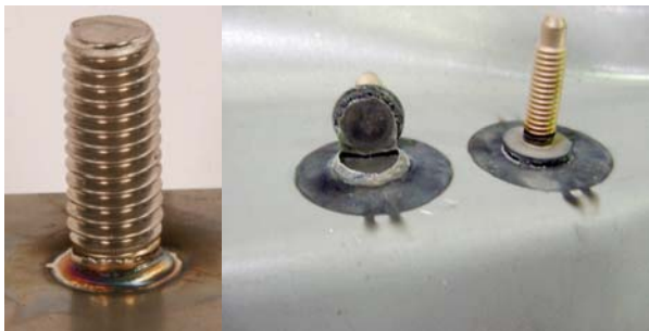
Fig. 6. 9.5mm diameter stainless stud short cycle welded without ferrule (left) and W-top welded to laminated steel (right)
