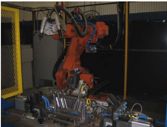
Fig. 1. Robot stud welding cell for the production of sheet metal parts
