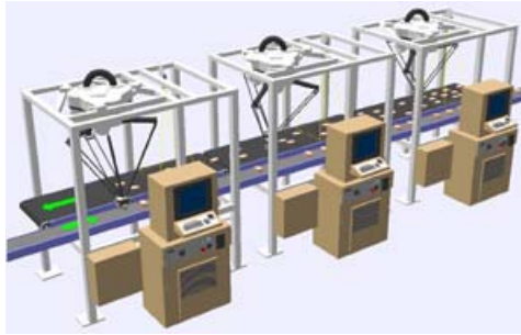
Fig. 2. Packing application using FlexPicker and vision system
