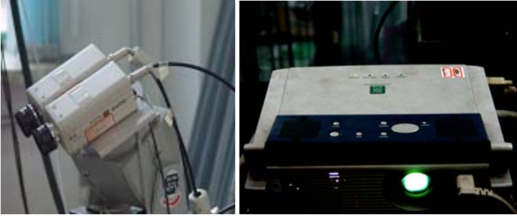
Fig. 2. The prototype system with two cameras (left) and a video projector (right)
