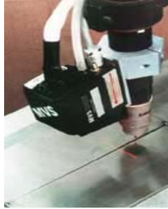
Fig. 1. Laser vision Seam Tracker™ from Meta vision systems ( www.meta-mvs.com )
