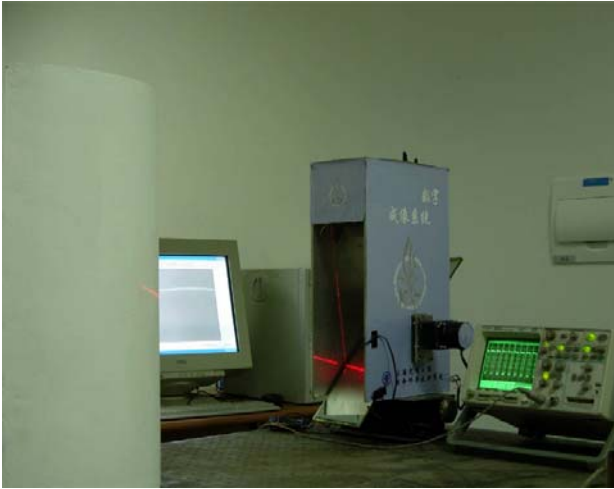
Fig. 3. Picture of the experimental apparatus: the proposed wide angle-of-view integrated vision system and the inspected model
