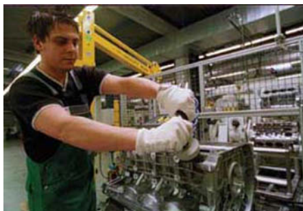
Fig. 5. Manual cleaning operations in a foundry plant
