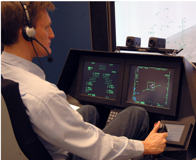
Fig. 2. Simulator tests for HCI research into Pilot Observing Avionics , using the Companion principle
