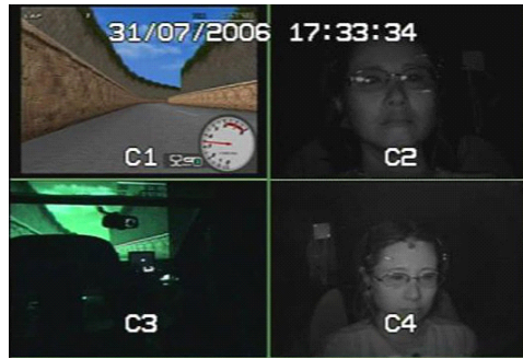
Fig. 1. Experimental settings. The upper left shows the driving image presented to the subject, the lower left is a rear view of the experimental system, and the two images in the right are subject's face images recorded by infrared CCD cameras.
