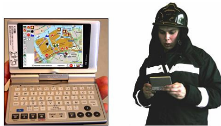
Fig. 1. Zaurus PDA ( left ) and the fireman user profile using the crisis multimodal adaptive system ( right )
