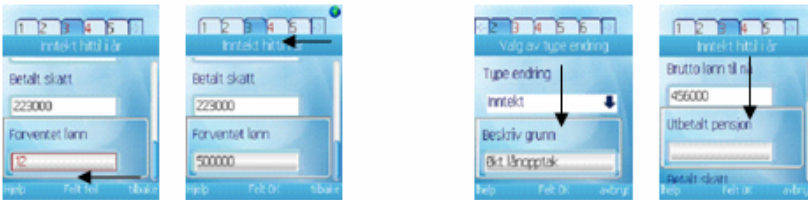
Fig. 4. Changes in the colour scheme indicate invalid input; input field containing ‘12’ and card number ‘4’ have changed colour (left). Working area is accentuated by a frame (right).
