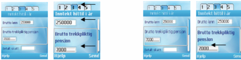
Fig. 5. Changes in font size all over the user interface (left), or only in selected fields (right)
