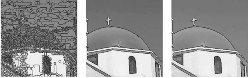
Fig. 11.8. Watershed partition, left , oversegmentation reduction by the algorithm [110], middle , and segmentation by the new algorithm, right
