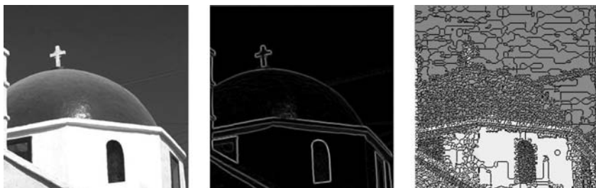
Fig. 11.3. A gray-level image, left , the gradient image, middle , and the watershed partition, right
