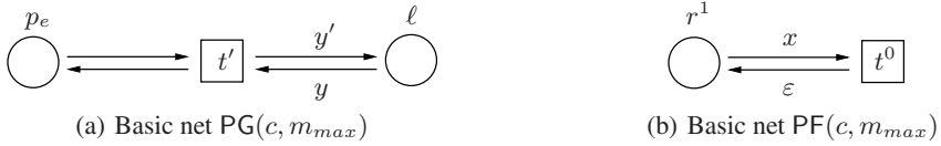
Fig. 5. Basic nets for packet generation and packet flush
