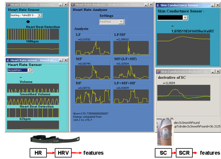
Fig. 4. Designed Real Time Heart Rate and Skin Conductance Emotional Feature Analyzer
