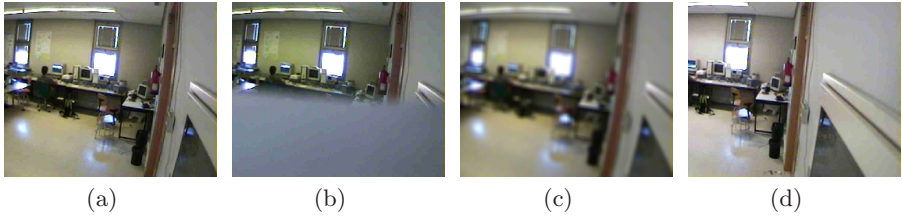
Fig. 2. Some examples of video camera sabotage. (a) No-sabotaged image. (b) Partial occlusion example. (c) Defocus example. (d) Displacement example.
