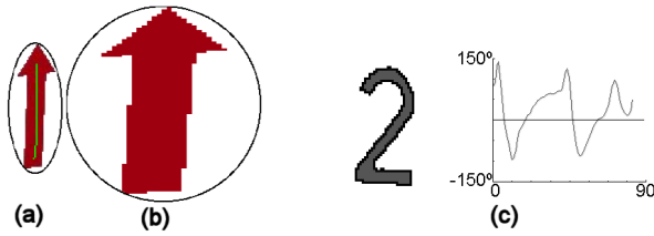
Fig. 4. a),b) Original and normalized curvilinear region; c)Curvilinear region shape and associated curvature function
