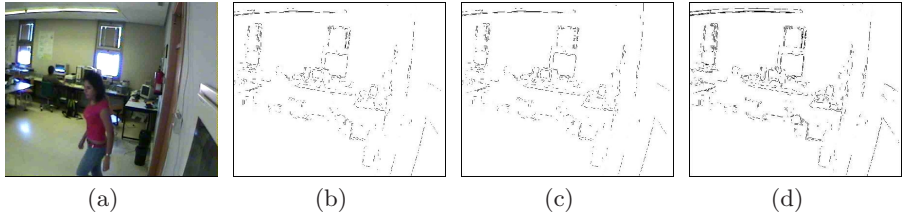
Fig. 3. Computation of the background model. (a): An image of the original sequence. (b-d) Background model after (b) 30 frames (1 iteration), (c) 60 frames (2 iterations), (d) 120 frames (4 iterations).
