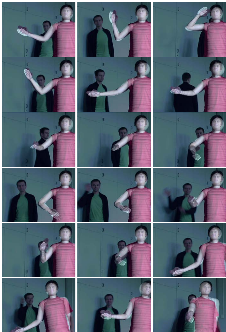
Fig. 8. Result sequence with dynamic background. The estimated model pose is overlaid on the original camera image. Ten DOF were estimated.
