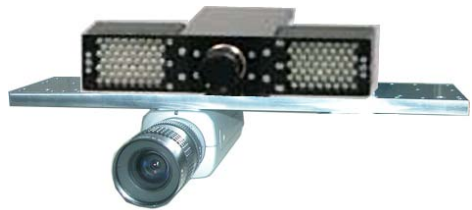
Fig. 5. Setup used for the arm tracking. PMD camera on the top with IR-LEDs next to it.
