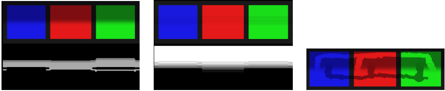
Fig. 2. Results trying to remove the shadow from a synthetic shadow image. [Left] Image (top) and detected shadow edges (bottom). [Middle] Estimated shadow free image (top) Estimated \alpha (bottom) Black is \alpha = 0 and white is \alpha = 1 . [Right] Augmented shadow image.
