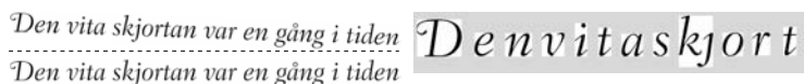
Fig. 5. Top left: Example of an input image. Bottom left: Input image after rotation. Right: 12 first sub images after segmentation.
