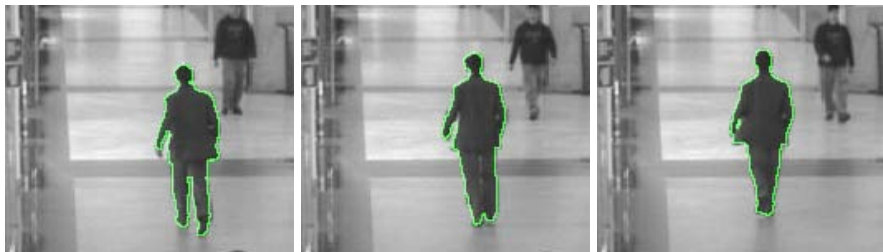
Fig. 1. Segmentation of a person in human walking sequence using the classical Chan-Vese model
