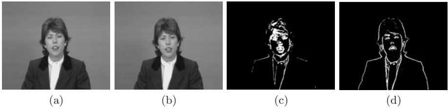
Fig. 5. (a) and (b): Two successive frames of an image sequence showing a moving speaker-woman. (c) and (d); Moving and static boundary detection using our system.
