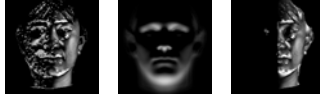
Fig. 4. The first image is the original needle map projected to the image plane. The second image is the mean needle map that we use as the template. The third image is the needle map projected to the image plane after the Mean Needle Map Alignment (Sect. 2). The third image compensates the concave/convex problem of the first one.
