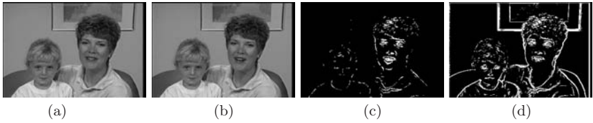
Fig. 6. (a) and (b): Two successive frames of an image sequence showing a moving woman and a child. (c) and (d); Moving and static boundary detection using our system.
