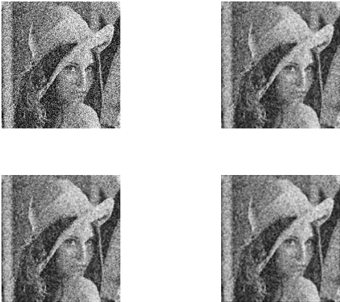
Fig. 2. Top left: degraded image with Gaussian noise (0 mean, 0.05 variance), top right: adaptive Wiener filter, bottom left: mean filter, bottom right: double adaptive filter
