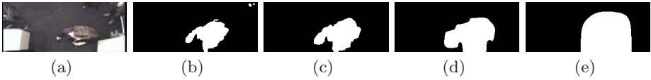
Fig. 5. Results obtained from one sequence by only changing the spatiotemporal blocks size. (a) Input sequence. (b) b = 16 . (c) b = 32 . (d) b = 64 . (e) b = 128 .
