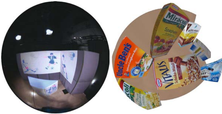
Fig. 3. Examples for fisheye images (scene registration). Left: real fisheye image. Right: synthetic image.
