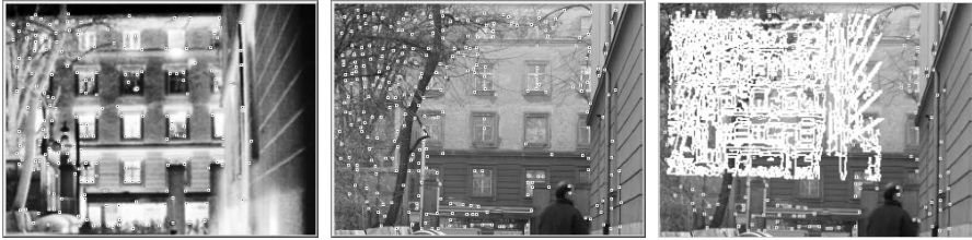
Fig. 5. An example of very problematic image. The corners in IR (left) and RGB (middle) images are also shown. The “registration” is obviously worthless.
