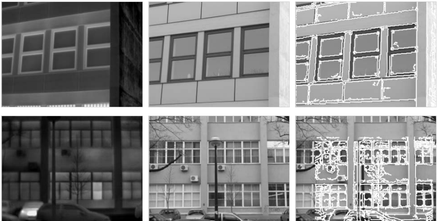
Fig. 4. Subjective evaluation of the registration. The rightmost images are obtained by laying the edges from IR images (leftmost) over the RGB images (middle).
