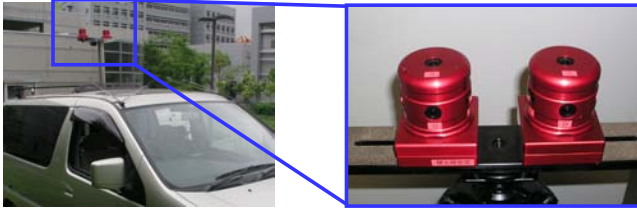
Fig. 2. Omni-directional multi-camera systems mounted on a vehicle
