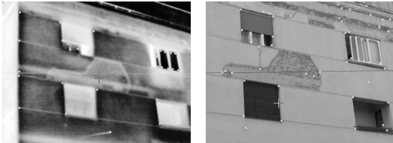
Fig. 2. Corners detected in IR (left) and RGB (right) images by using Harris corner detector
