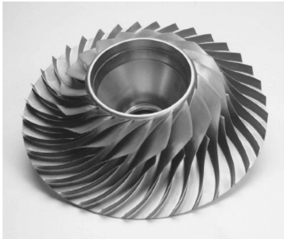
Fig. 6.13. Impeller used in a small engine for regional jets, Ti-6242, bi-modal microstructure (courtesy J. A. Hall, Honeywell Engines and Systems)
