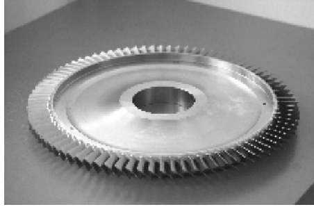
Fig. 6.14. High pressure compressor blisk used in the EJ 200 aero-engine, IMI 834, bi-modal microstructure (courtesy D. Helm, MTU)
