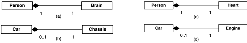
Fig. 2. (a-b) Wholes and their Essential parts; (c-d) Wholes and their Mandatory parts
