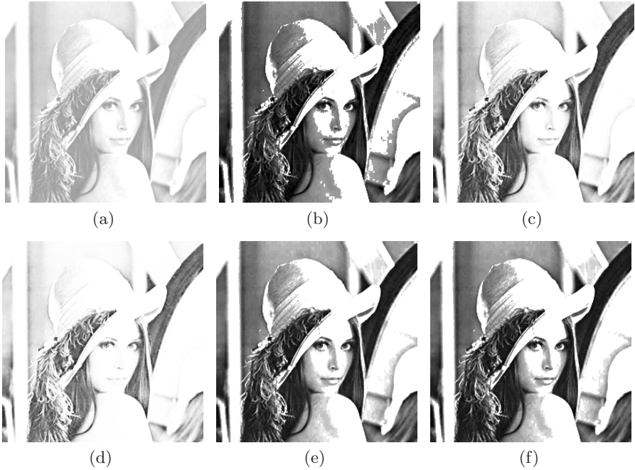
Fig. 5. (a) Over-exposed gray-scale image and images obtained using (b) the histogram equalization technique and the IFIP framework employing entropy (c) E_1 ( \lambda_{opt} = 1.60 ), (d) E_2 ( \lambda_{opt} = 2.72 ), (e) E_3 ( \lambda_{opt} = 0.59 ), and (f) E_4 ( \lambda_{opt} = 0.45 )
