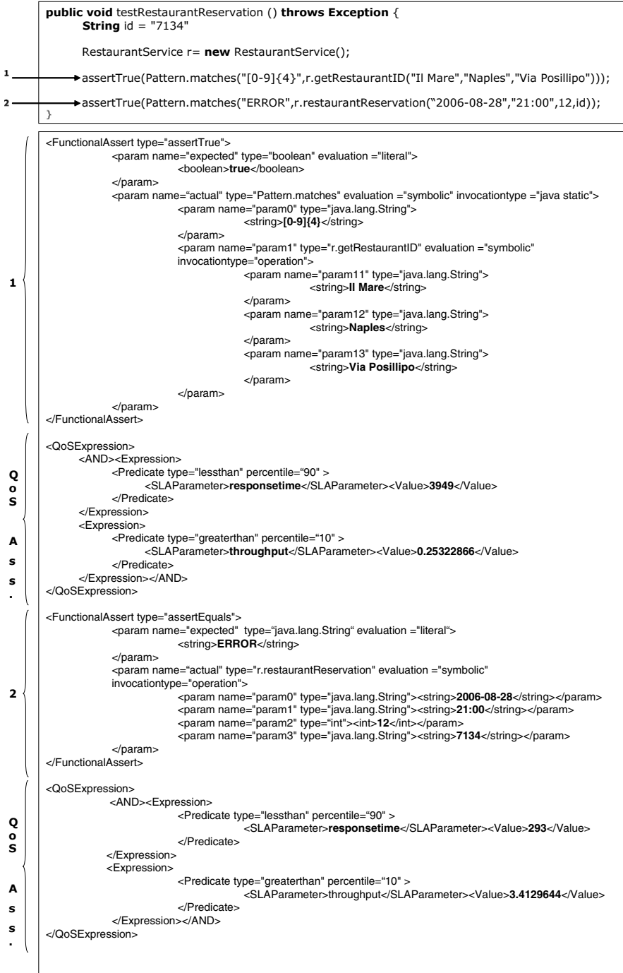
Fig. 8.4. Mapping of a JUnit test case onto a XML-encoded service test case
