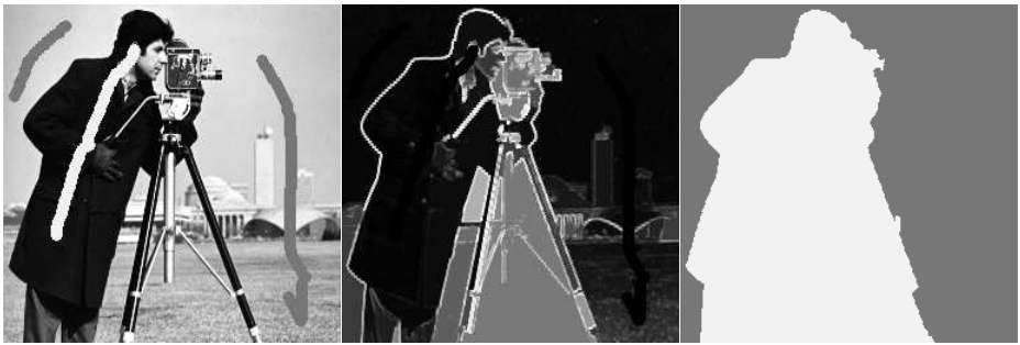
a) 3 markers placed on the cameraman image b) result of the swamping of the gradient, this image has three minima c) resulting segmentation
