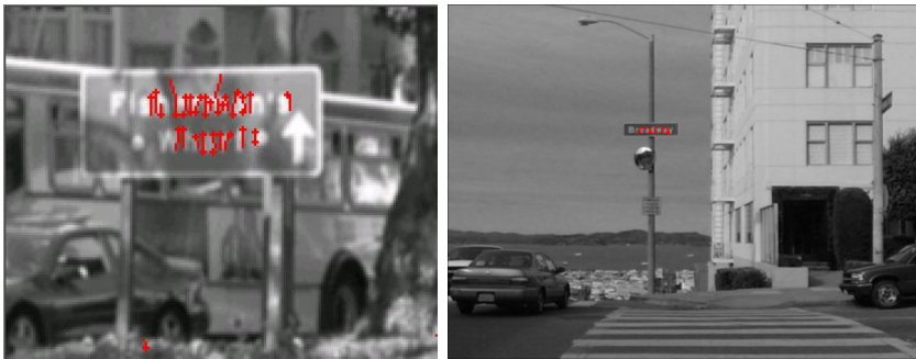
Fig. 4. Experimental results. Left, text segmentation from Fig. 3(b) demonstrating robustness to non-uniform lighting. Right, result demonstrating performance in high clutter.
