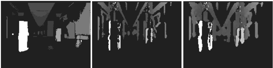
Fig. 5. Disparity Map Results: On the left side our method, on the center side the SSD, and on the right side the SSD multi-scale
