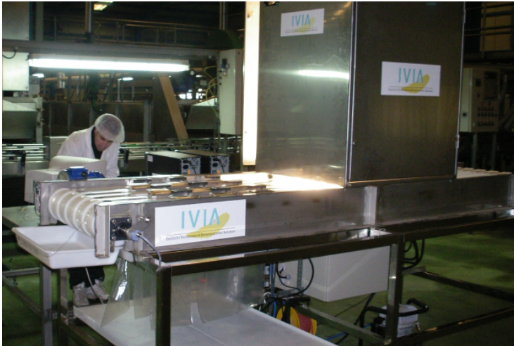
Fig. 1. Prototype for the automatic sorting of satsuma segments
