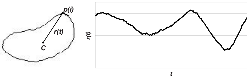
Fig. 5. Polar signature of the boundary of the segment
