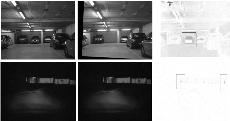
Fig. 2. Registration of corresponding frames. From left to right: frame of first video, warped frame of the second video and contrast inverted difference.
