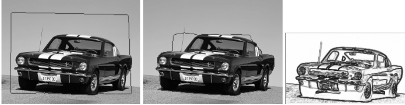
Fig. 4. An application with a coincidence percentage: a) Initial contour; b) 75% of coincidence; c) Gradient image
