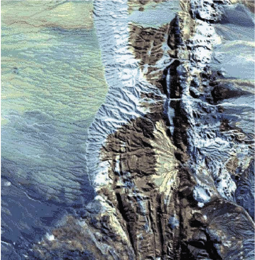
Fig. 8.3 Indexed color image using a colormap containing 16 different colors. The result is displayed using imshow . Original image courtesy of NASA/GSFC/METI/ERSDAC/JAROS and U.S./Japan ASTER Science Team.
