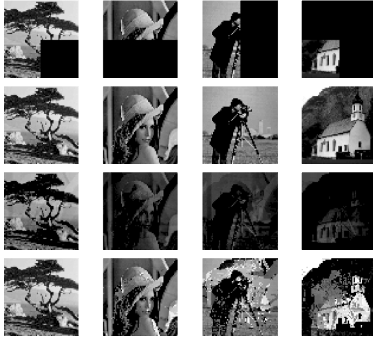
Fig. 8.2. The images in the top row represent severely incomplete versions of original face images. The following rows show - from top to bottom - the corresponding recalled patterns using the morphological memory W_{XX} , the OLAM, and the generalized BSB model
