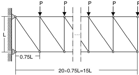
Fig. 1. 20-floor cantilever truss structure
