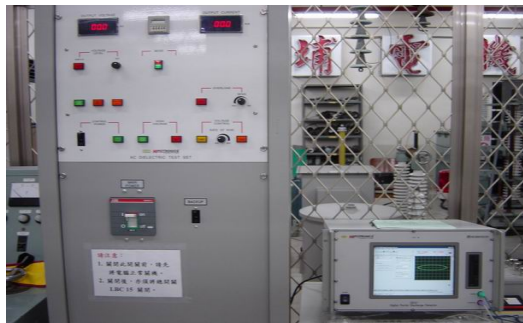
Fig. 3. PD analyzer and control panel
