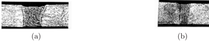
Fig. 4. The photos for the cross section of the welding seams: (a) IF (X60) and (b) WLZn (X60)
