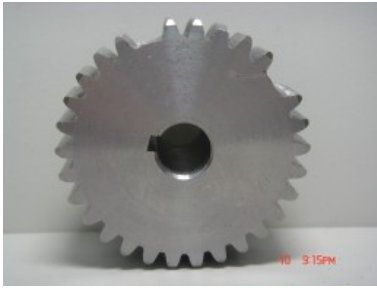
Fig. 5. Tooth breakage gear
