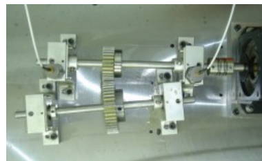
Fig. 4. Shaft not parallel of gear system
