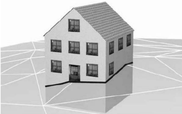
Fig. 3.3 CityGML’s ‘TerrainIntersectionCurve’ (shown in black), a 3D polyline representing where the building meets the terrain. Source: [8]
