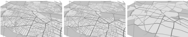
Fig. 21.5 Generalized cells for three degrees of generalization (no outlier handling)
