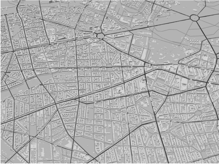
Fig. 21.2 Snapshot from the visualization of part of the 3D city model of Berlin containing approx. 60,000 3D building models and approx. 6,500 streets without generalized building models)
