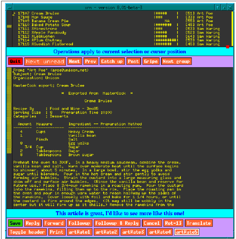
Fig. 2. A modified Xrn news reader. The GroupLens project added article predictions (lines of 0-9 #s on the top right) and article rating buttons (bottom)
