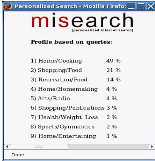
Fig. 2.7. A conceptual user profile representing a user interested in cooking, built from the top 3 levels of the ODP and the user's search history
