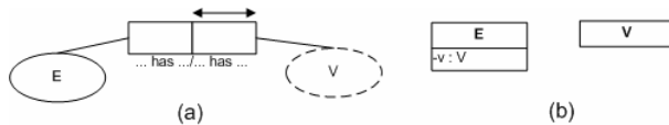
Fig. 3. (a) Internal uniqueness constraint on one role value type role of binary fact type, (b) resulted UML model
