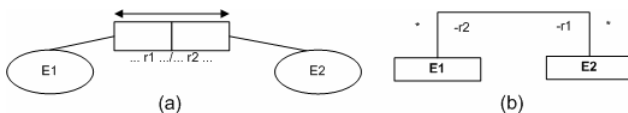
Fig. 4. (a) two role internal uniqueness constraint on binary fact type, (b) resulting UML model
