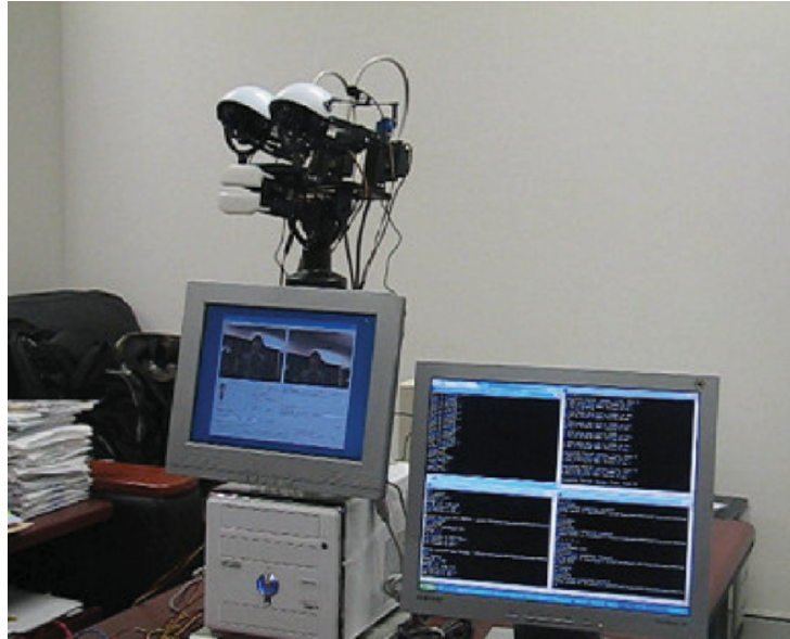
Fig. 2. Artificial Brain with two eyes, two ears, and one microphone. The lips are used for lip-sink, and 2 LCD displays are used for camera inputs and internal processor status
