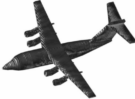
Fig. 7: Surface currents (at 500 MHz) on an airplane illuminated by a plane wave
