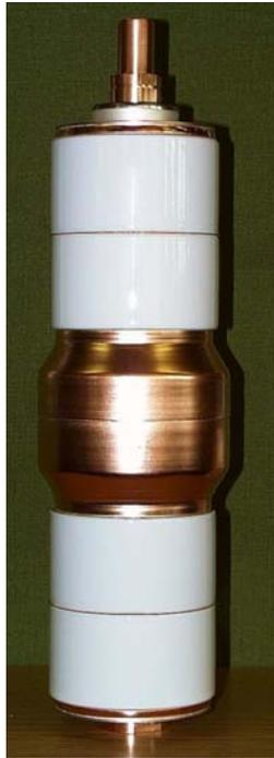
**Fig. 9.11.** High voltage vacuum interrupter (prototype): for 72.5 kV and 31.5 kA; 150 mm tube diameter; 500 mm length
