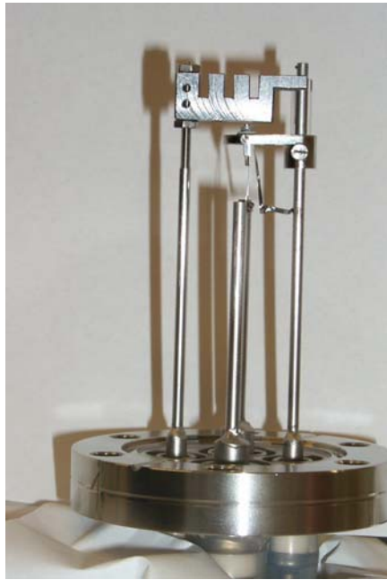
Fig. 10.42. UHV diode emission test flange with a 0.65 W I cathode unit below the Ta anode on top, as used by Philips Research (courtesy of Philips Research Aachen)
