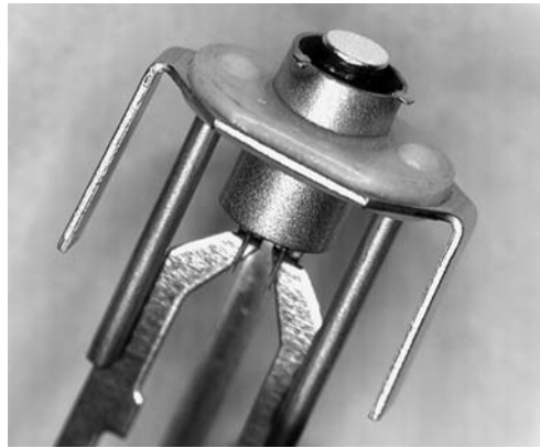
Fig. 10.14. Philips 0.65 W oxide cathode unit for CRTs
