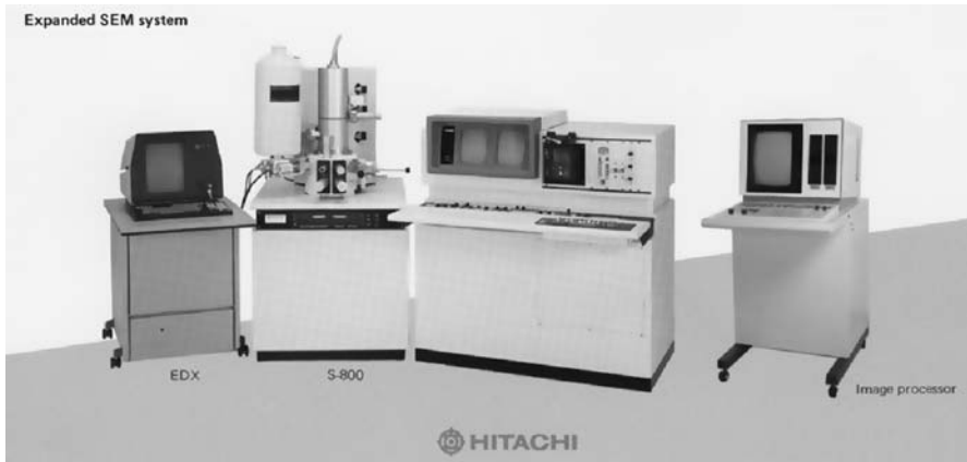
Fig. 4.53. Field emission SEM system with energy dispersive X-ray spectroscopy and image processing unit (courtesy of Hitachi)
