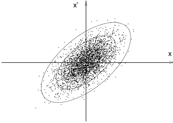
Fig. 8.16. Simulated Gaussian phase space distribution in the coordinates x, x' . The ellipses for one, two and three standard deviations are indicated
