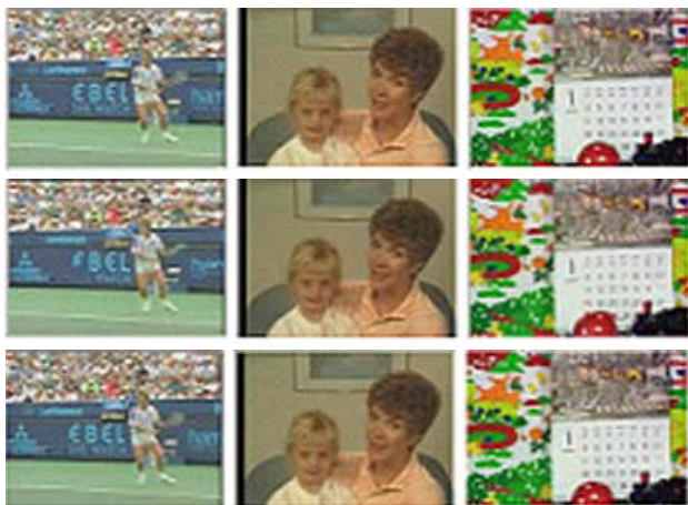
Fig. 8. Examples of the reconstruct images with MPEG-4, ICA-based, and selective ICA-based algorithms. (a) MPEG-4 baseline, (b) ICA-based method, (c) Selective ICA-based method (Threshold = 2).
