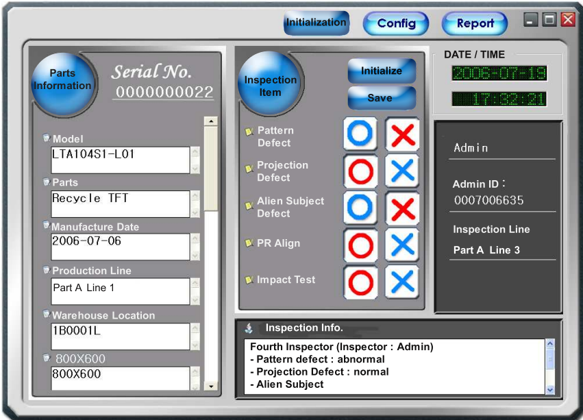
Fig. 4. Main screen for parts inspection
