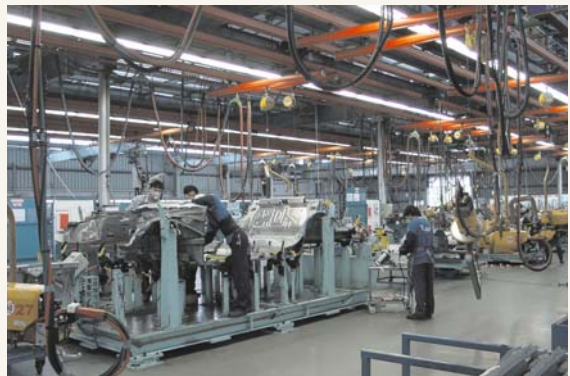
Fig. 2.28: Mounting body parts prior to welding using handheld clamps
