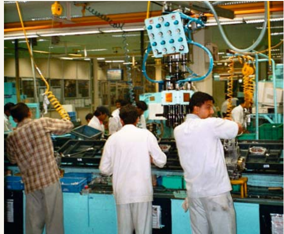
Fig. 5.11: Manual assembly of motorbike gearboxes at Hero Honda in Gurgaon, India
