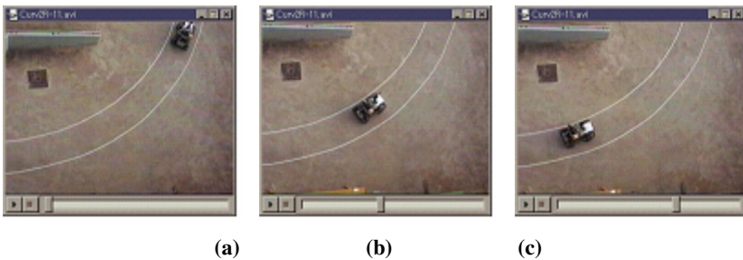
Fig. 8. Visual guidance test on curved guideline. (a) at the starting (b) at the midway (c) at the finishing.
