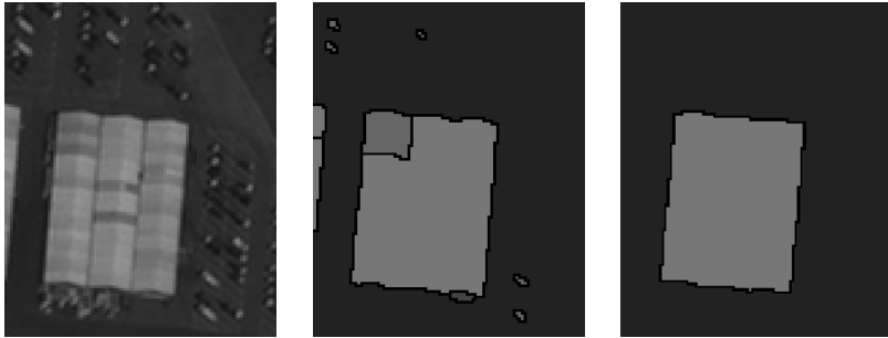
Fig. 11. Left: Industrial building in IKONOS data, Middle: Vanhamel approach result at LYV optimum, Right: Our result at LYV optimum
