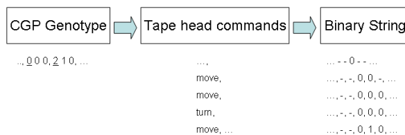
Fig. 3. The three step procedure for producing a GA bit-string from the CGP genotype, via a set of tape head commands
