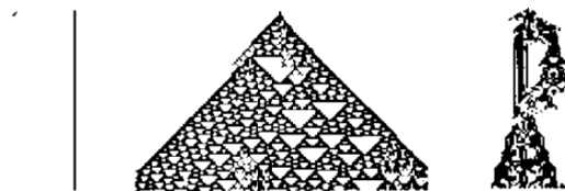
Fig. 1.45. Evolution of small initial perturbations in CA, as shown by the difference (modulo two) between patterns generated from two disordered initial states differing in the value of a single site. The examples shown illustrate the four classes of behavior found. Information on changes in the initial state almost always propagates only a finite distance in the first two classes, but may propagate an arbitrary distance in the third and fourth classes (adapted from [Wol02, Wol84]).
